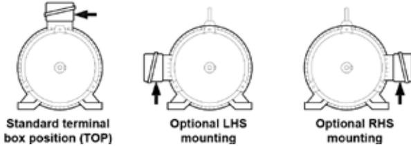
Conduit entries for motors are provided tapped, with thread details set out below.
