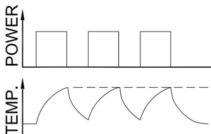
**S7 Continuous periodic duty with starting and electric braking**
