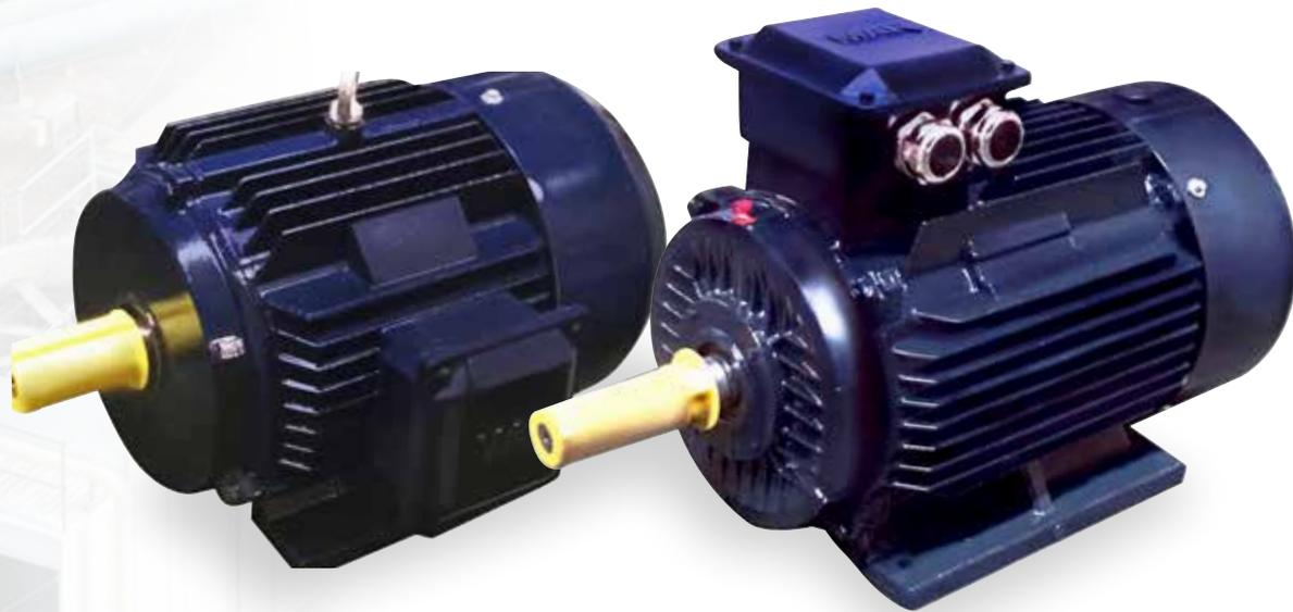
**The CDA series is a range of totally enclosed fan cooled (TEFC) cast iron construction motors built for general industry application with IEC®\* frame sizes from 80 to 315 CENELEC frame allocation as standard.**
